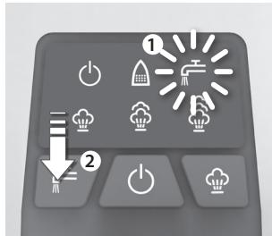
**7.** If the **low water level** indicator is illuminated (followed with two beep sounds), refill the water tank. After refilling the water tank, press and hold the refil reset button for about 6 seconds. The low water level indicator light will turn off. Steam can now be used again.
