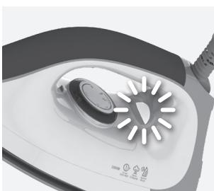
**5. When the temperature indicator light turns on,** the steam generator is pre-heating. When the light turns off, it is ready to be used. The hot soleplate indicator turns red when the iron reaches 40°C. Press the steam button to discharge a concentrated shot of steam. Then hold one more minute in order to clean the steam generating system.
