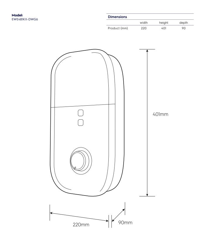
Please note! Dimensions to be used as a guide only. All customers MUST refer to the user manual supplied with the product for detailed installation instructions. © 2021 Electrolux S.E.A PTE. LTD. E\_DIM\_EWE481KX-DWG6\_Jun21
