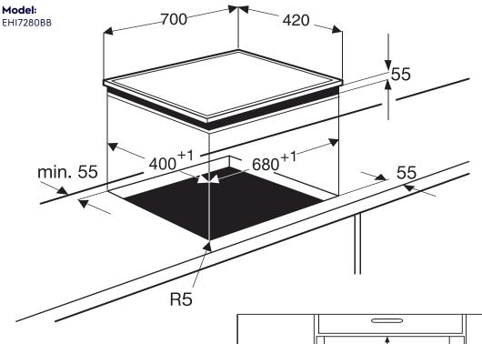
**Note:** The clearance must meet or exceed the minimum recommended for both the rangehood and cooktop. Refer to the rangehood installation manual
