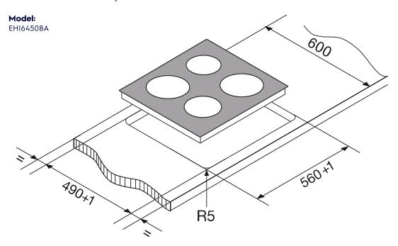
**Note:** The clearance must meet or exceed the minimum recommended for both the rangehood and cooktop. Refer to the rangehood installation manual
