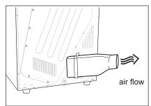
Inlet and outlet points need clear airflow to prevent overheating, so ensure there is adequate ventilation. (i.e. open window or external door.)
