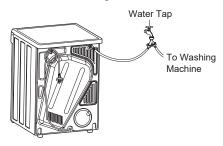
6. Turn on the water tap and check for leaks at all connection.
