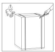
Remove the carton box. Remove the polystyrene packaging materials. Remove the plastic bag which cover the machine.
