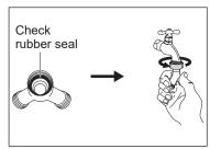
Connect the inlet hose for the washer and the dryer to the Y-Connector and tighten them.
