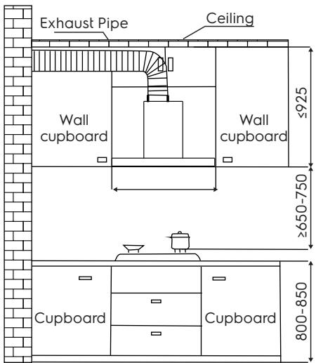
Exhaust Pipe Routing Through Ceiling
