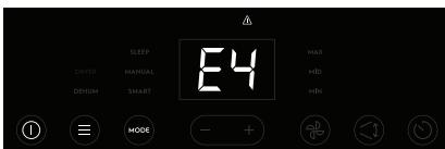
**E4-** DC Motor failure
