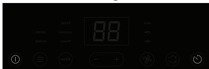
1. Tap (touch and release) "①" to turn on the appliance. The display shows the current room humidity. The DEHUM function and SMART mode are activated by default.
