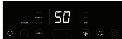
1. Tap "swing" button to enable the auto swing feature, the louvre will swing up and down automatically.
